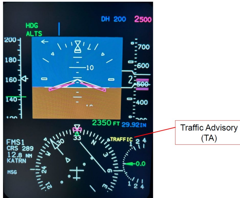
Figure 4 – Example of how a TA appears to pilots on an aircraft primary flight display
